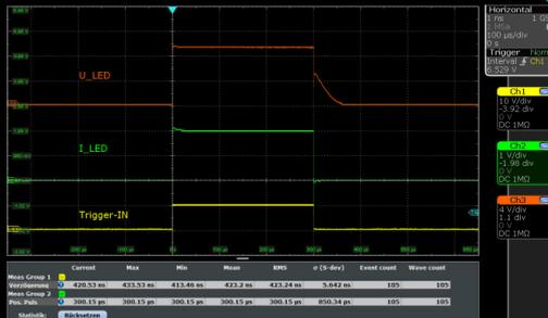
Fig. evotron DCC2404-1WS – 300 µs LED current pulse, time division: 100 µs
