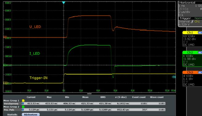
Fig. evotron DCC2404-1WS – 2 A LED current pulse, time division: 2  $\mu$ s
