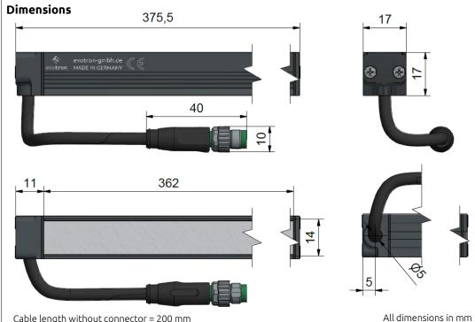
Cable length without connector = 200 mm
